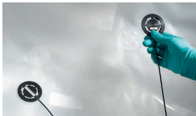
Fig 5. The optical sensor is embedded in the underside of the Cellbag bioreactor. Shown here is the bag adapter/optical fiber cable attached to the bag port.
