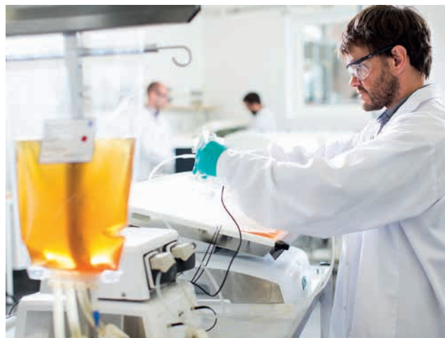
Fig 3. Cellbag bioreactor equipped with ReadyMate connectors facilitate quick aseptic connection to downstream operations.
